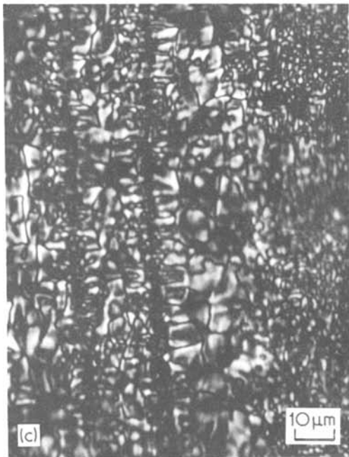
Figure 6 Nylon 11, tensile impact test, fractured at room temperature. (a) and (b) Scanning electron micrographs of fractured surface; (c) Photomicrograph of cross-section (transmitted polarized light).
