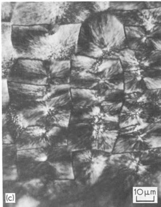
Figure 9 Nylon 12, tensile impact test fractured at room temperature. (a) and (b) Scanning electron micrographs of fractured surface; (c) Photomicrograph of cross-section (transmitted polarized light).
